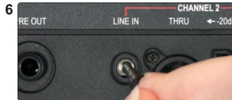
For a stereo signal from an MP3 player, attach 1/8" stereo cable into the Channel 2 1/8" input.
