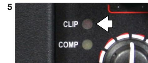
Reduce the Input Levels if the Clip LED comes on.
