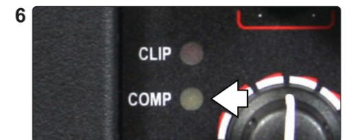
Max. level is reached when the yellow "Comp" light only flashes at peak levels. If the light is on constantly, turn the level controls down to avoid damage to the PA6S.
