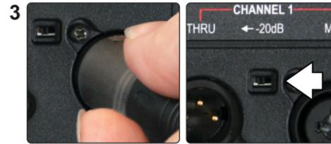
For a balanced mic signal, plug the XLR male end of the cable into the XLR/1/4" Combo Input on the PA6S. For strong signals, engage the -20dB Pad Switch to prevent distortion.
