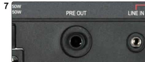
The Pre Out provides a Line Level mix of both channels.
