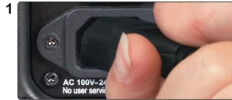
Connect power cable to PA6S, connect other end to a power outlet.
