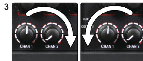
Level control: turn clockwise to raise the level. Turn counter-clockwise to lower the level.
