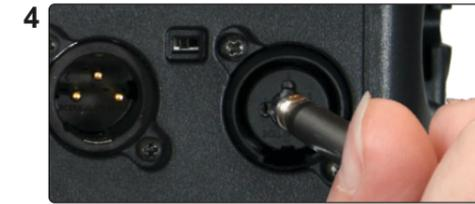
For Balanced or Unbalanced Line Level, plug the 1/4" cable into the XLR/1/4" Combo Jack on the PA6S.
