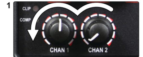
Ensure that both channels have their levels lowered by turning counter-clockwise.
