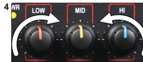
EQ controls - Low/Mid/Hi: To increase the low, mid, and high frequencies, turn the appropriate tone control clockwise. To decrease, turn counter-clockwise.
