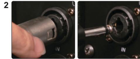
2 From your mixer or source, connect an XLR or 1/4" Cable into the Combo Jack Input located on the back of the GPS-8.
