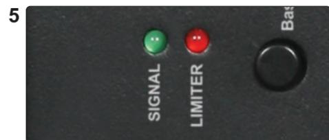
5 The green signal LED indicates you have input signal. The Red Limiter indicates too much signal. If lit, turn the input down.
