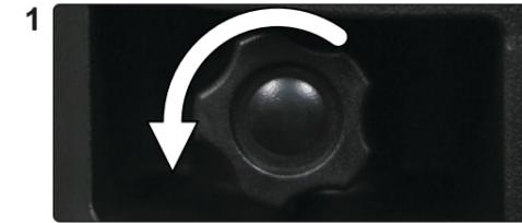
1 Loosen the knob on the back of the GPS-8 by turning counter-clockwise to ensure there is no obstruction in the mounting hole from the fastener.
