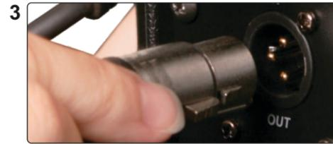
3 To loop to a second GPS-8, connect an XLR female into the output and the male end of the cable to the input of the second GPS-8.
