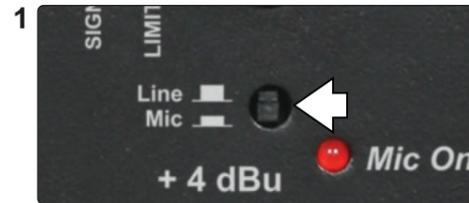
1 For Line Level input, the button should be in the up position. For Mic Level input, press the button in, the Mic On LED will light up.
