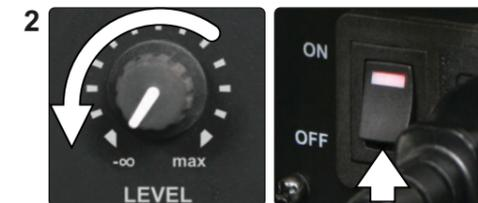
2 Insure the input level control is turned down (fully counter-clockwise) Turn the power switch on.
