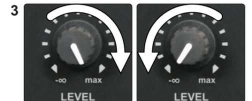
3 Level control: turn clockwise to raise the level. Turn counter-clockwise to lower the level.
